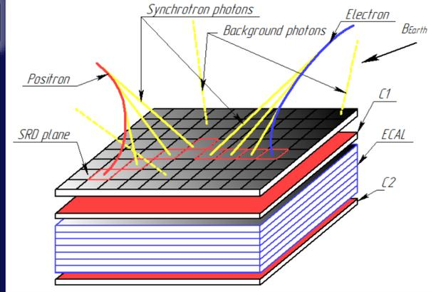
Fig. 3 Scheme for registering positrons and electrons using synchrotron radiation
