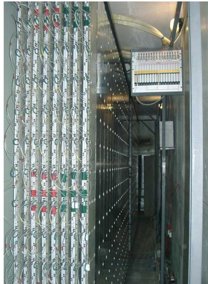
Each SM has an effective area  $8.4 \text{ m}^2$  and consists of 8 vertical planes of streamer tube chambers. The length of the chambers is 3.5 m, inner tube cross section is  $9 \times 9 \text{ mm}^2$ . The planes of the chambers are equipped with a two-dimensional system of external readout strips.
