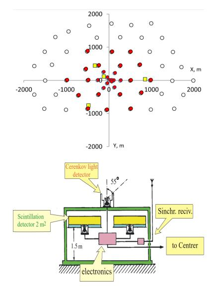
The Yakutsk array studies cosmic rays in the energy range above 10 PeV. The main parameter obtained from the measured data is  $S_{600}$  – the density of particles at the shower core distance 600 m.
