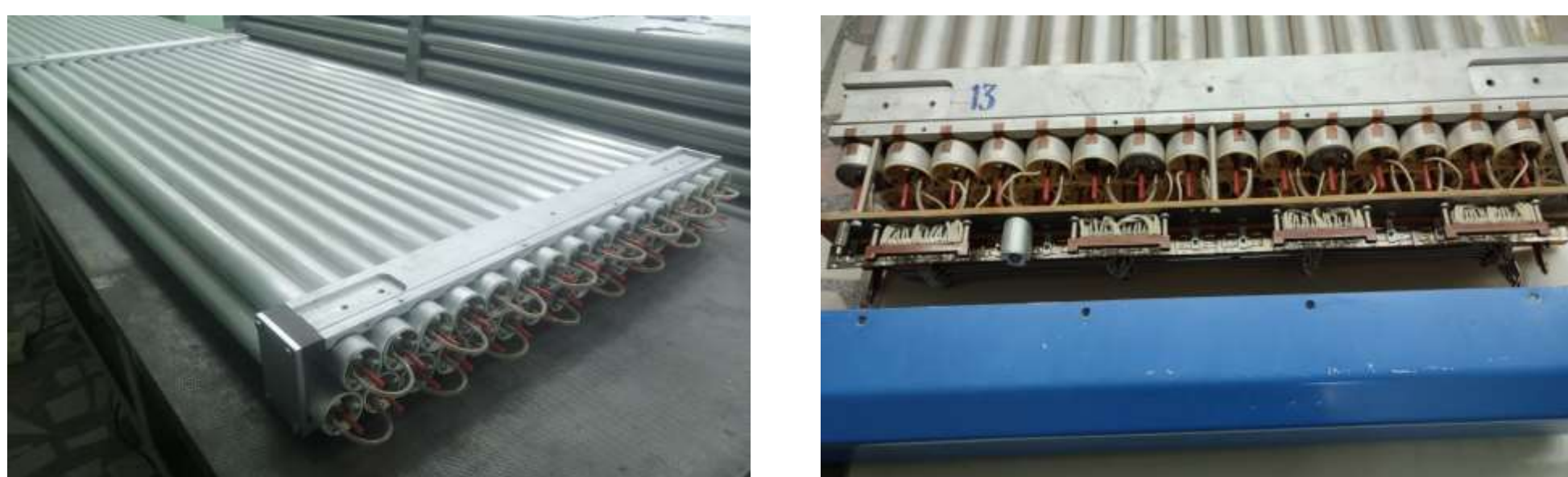
Fig. 4. Module of 32 DTs, view from two ends
