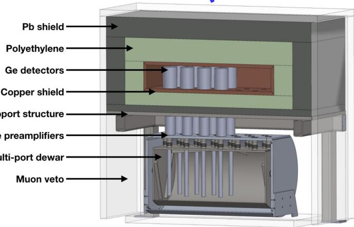
16 kg of HPGe detectors for CEvNS measurement
