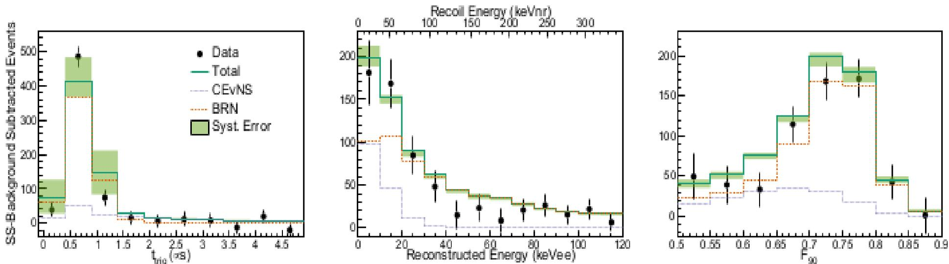
Projection of the best-fit maximum likelihood probability density function (PDF) from A (top) and B (bottom) Analyses on  $t_{\text{trig}}$  (left), reconstructed energy (center), and  $F_{90}$  (right) along with selected data and statistical errors. The fit SS background has been subtracted to better show the CEvNS component
