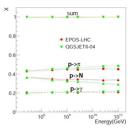
Most crucial energy transfer, p->γ, is energy independent and about same in two generators. Same for p->h transfer.
