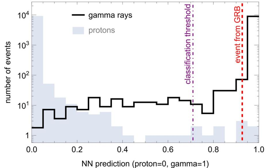
Predictions distribution of the gamma-ray – proton classifying neural network. The values of the classification threshold (0.71; dot-dashed line) and of the prediction for the event analyzed in this work (0.927; dashed line) are shown.
