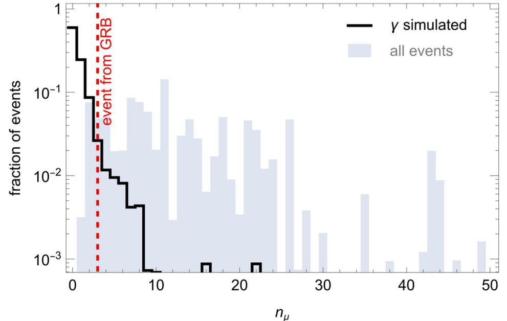
To estimate the hadron background, we used data selected from the same arrival direction ( $\theta$ ,  $\varphi$ ) in which the gamma-ray burst is located. Then we weighted the events taking into account the log-normal distribution with the mean value corresponding to the  $N_e$  event. A double Gaussian distribution by arrival angles was also added. Taking these weights into account, we construct distributions of the selected events by the number of muons  $N_\mu$
