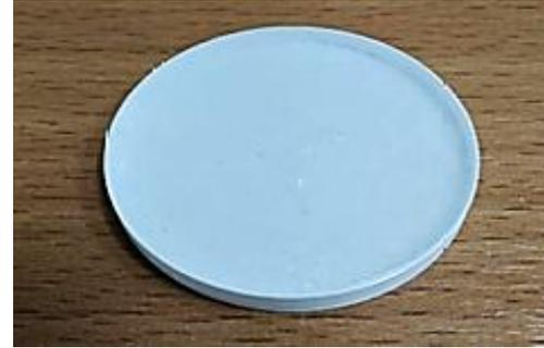
Dispersed (heterogeneous) scintillators with 35%  $^6\text{Li}$ -glass and silicone compound
